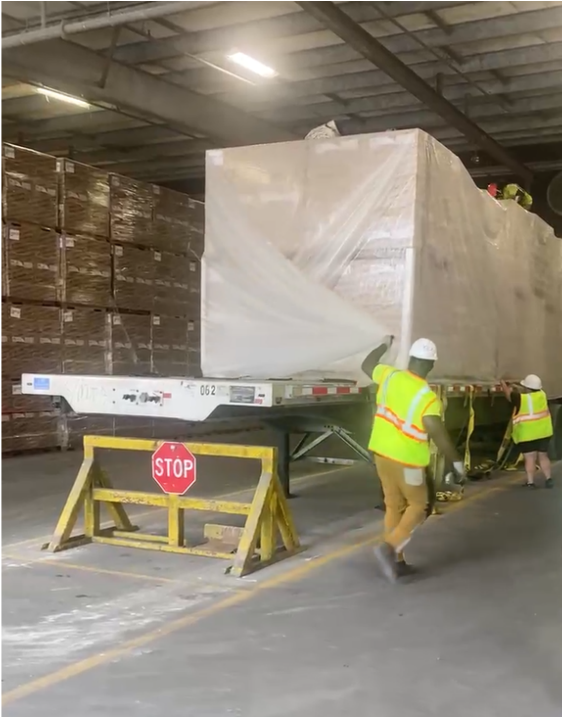
3. Load will be tarped and straps will be placed over the tarp with edge protection.
