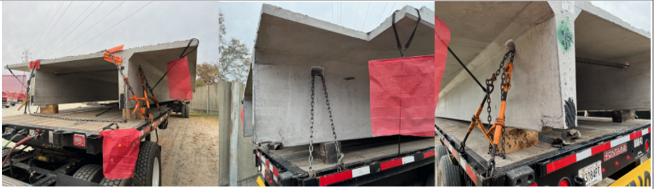
Figure 1: 35,000lb Double T secured with four chains. All four chains pass through the conduit pockets on the vertical faces of the t's. Use only conduit pockets located directly above supporting dunnage.
