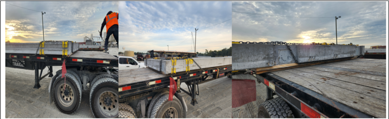
Figure 1: 35,000lb Metrodeck secured with four chains. Two chains at the front and two chains at the rear above the dunnage. Chains must be located directly above supporting dunnage. The trap chain is placed across the face of the product to prevent forward motion.
