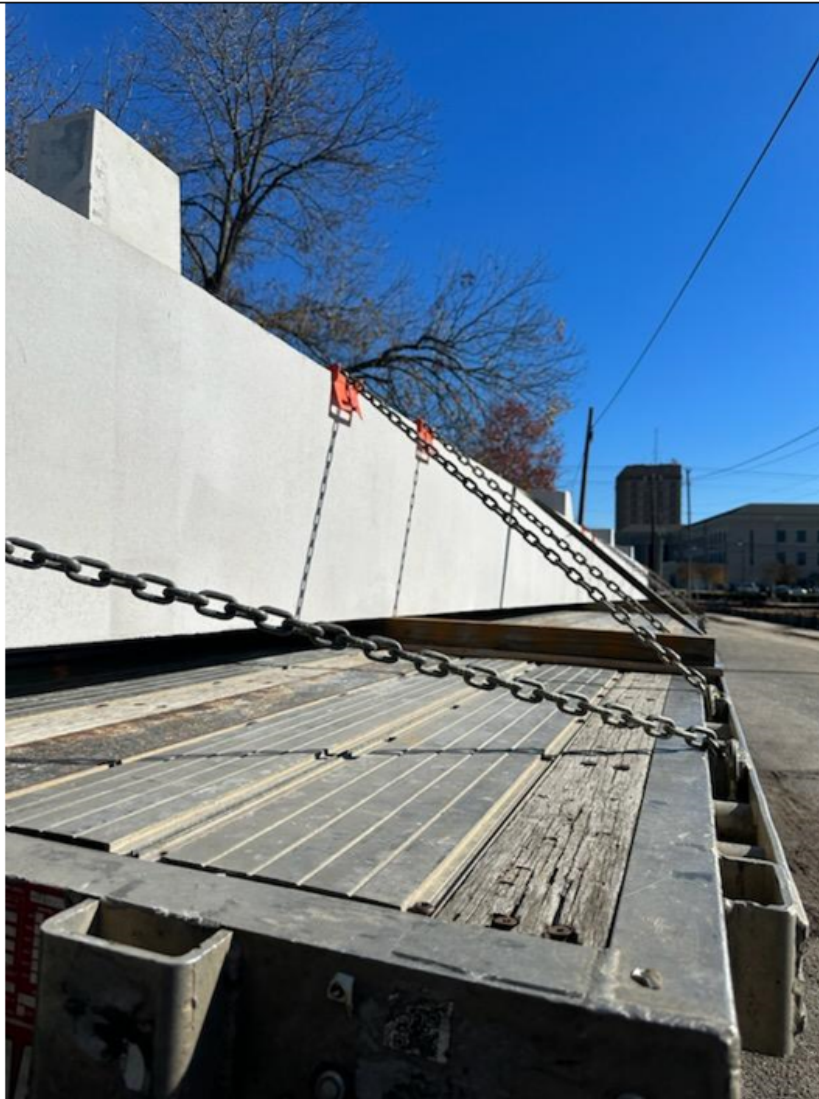
Figure 1: A precast column with a trap chain over the dunnage points, it also demonstrates the use of a trap chain to prevent forward motion.
