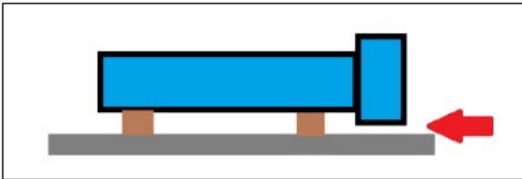
Figure 6: Bell pipe sitting on dunnage (brown) to keep the bell off the trailer deck. The red arrow showing the spacing between the bell and deck.
